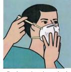
Cup the respirator in your hand. Hold the respirator under your chin with the nose piece up. The top strap (on single or double strap respirators) goes over and rests at the top back of your head. The bottom strap is positioned around the neck and below the ears.
